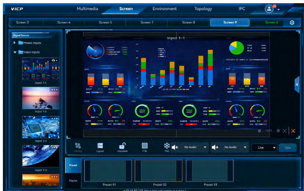
Figure 7-11 Screen control interface
